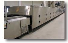
biscuit and cookie products. Control of the exhaust, air temperature and circulation velocity allow the operator to control the product moisture removal for maximum quality assurance.
